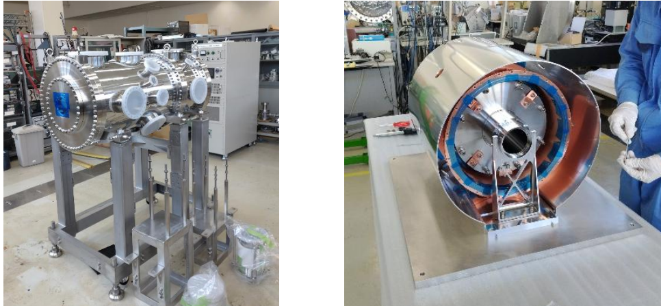
Figure 1. A vacuum chamber (Left) and a cryogen-free 5 T superconducting magnet (Right) for NIFS-EBIT.
