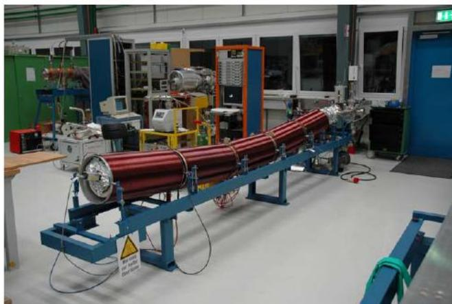
NEG coating facility commissioned. First sector equipped with new, coated chambers.
