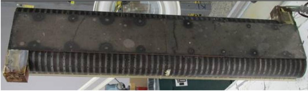
**Figure 6:** ANL's 0.5-m-long Nb<sub>3</sub>Sn model (prototype) magnet after the reaction and epoxy impregnation.
