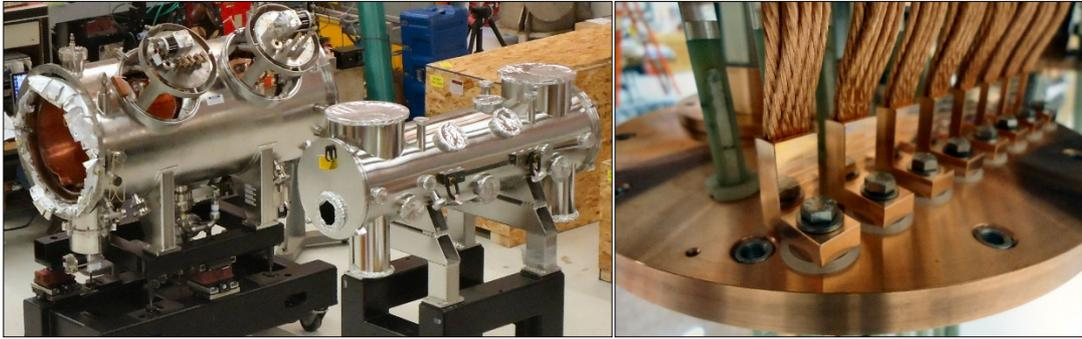
**Figure 6:** (left) comparison of original SCU vacuum vessel with smaller 2<sup>nd</sup>-generation vessel; (right) detail of corrector magnet current lead assembly.
