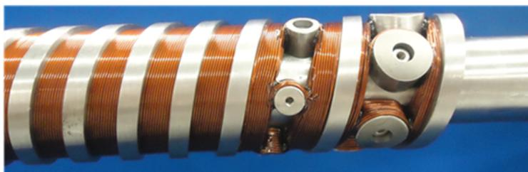
**Figure 12:** The 0.3-m-long, 31.5-mm-period prototype HSCU after winding.
