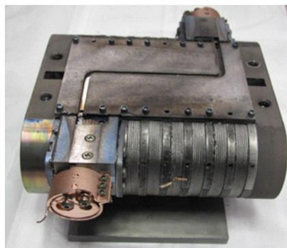
**Figure 23:** A picture of a short model magnet #6 (SMM6) after winding and reaction before the epoxy impregnation.
