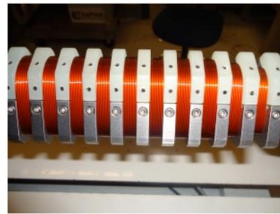
**Figure 20:** SCAPE core winding.
