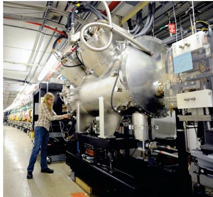
**Figure 1:** Superconducting undulator SCU18-1 installed in the APS storage ring.
