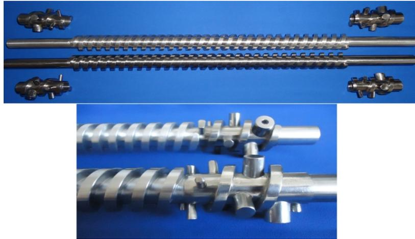
**Figure 11:** Top: Al and 1020 steel, 20-mm-period prototype HSCU mandrels with the turn-around structures not installed. Bottom: One end of the prototypes with the turn-around structures installed.
